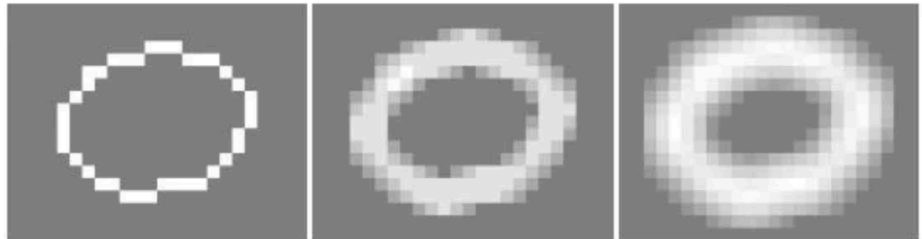
Figure 1: Example of “submanifold” dilation. Left: Original curve. Middle: Result of applying a regular 3 \times 3 convolution with weights 1/9 . Right: Result of applying the same convolution again. The example shows that regular convolutions substantially reduce the sparsity of the feature maps.
